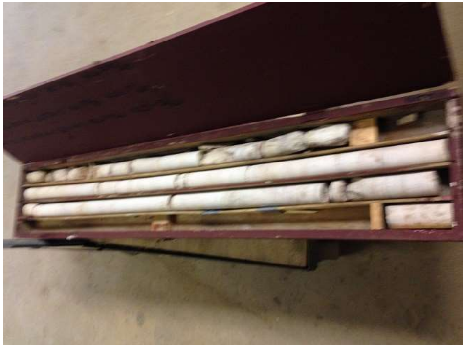
Photo 6: Exhibit D-6: Rock Core from WTG 31/Met 31C
