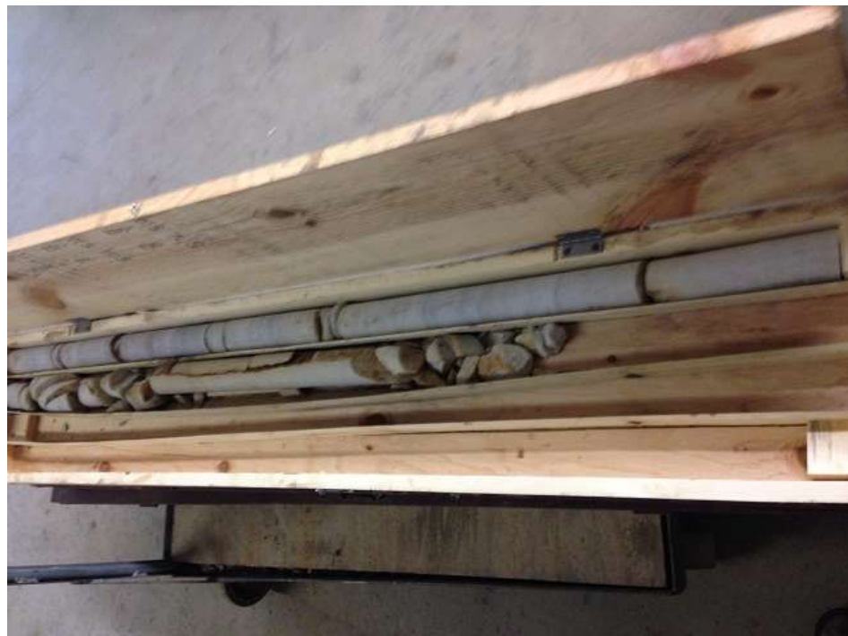
Photo 2: Exhibit D-2: Rock Core from WTG 36 (bottom)
